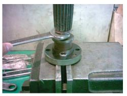
**Step 4.**Apply Loctite 554 sealant on the screw of oil filter flange. Install new oil filter onto oil filter flange and tighten it using a torque wrench with torque, 62 ft lb(850 kg-cm).
